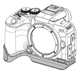
Install the camera onto 1) the expansion baseplate for Canon R10. Use ② the flat head screwdriver to install the tie down screw to secure the camera.
