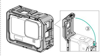
Press the power button  $\odot$  and open the side flip cover  $\odot$ . Place the action camera into the full cage, and close the flip cover  $\odot$  to complete the assembly.
