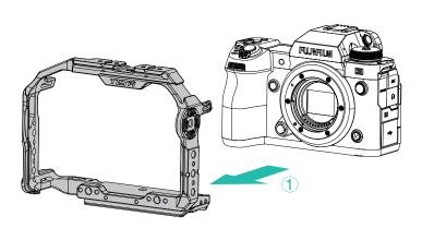
1. Place the camera into the ① X-H2S full cage. Take out the ② flathead screwdriver from the bottom of the cage. Tighten the locating screw ③ and the flathead screw ⑤ into the mounting threads at the bottom of the cage to complete the assembly.
