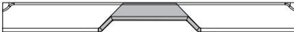
Sliding adjustment [bottom] Slides forward and backward for mounting wireless video unit.
