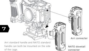
The cage is equipped with 1/4, 3/8 screw holes and Arri standard location holes.
