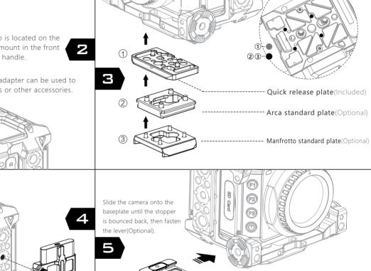
Install the Z-CAM E2-S6 camera into the cage then fasten the screws.Mount the camera in the correct position and then insert and tighten the mounting screw.
