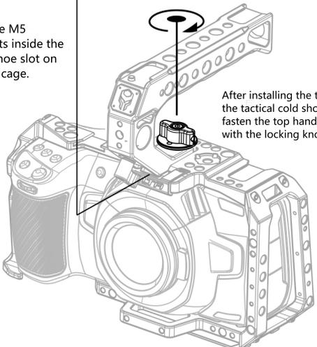
After installing the top handle into the tactical cold shoe mount, fasten the top handle to the cage with the locking knob as shown.
