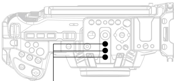
There are three M5 mounting ports inside the tactical cold shoe slot on the top of the cage.
